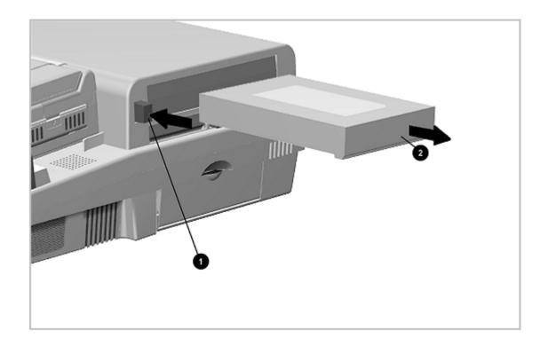
Figure 7-4. Removing a Battery Pack from a MultiBay
